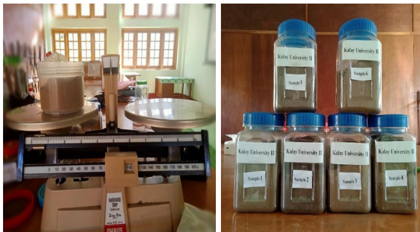
Figure 4 Photograph of weighing soil samples with 100grams and the collection and preparation of fine soil samples.
