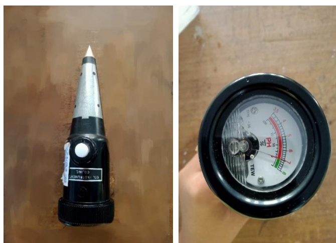
Figure 5 Photographs of Kelway Soil Acidity and Moisture Tester
