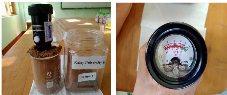
Figure 6 Photographs of measured the pH (potential hydrogen) of soil sample.
