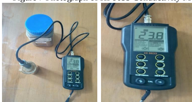
Figure 8 Photographs measuring the conductivity of Kalay University's soil sample
