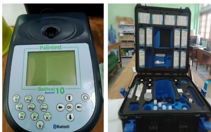
Figure 9 Photographs of Soiltest 10 photometer and Chemical box
